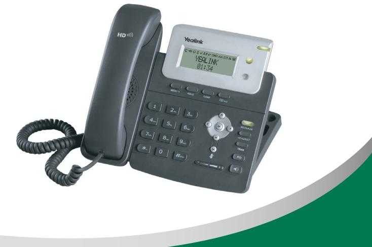
Yealink expands its lineup of IP phones with a new entry-level product SIP-T20P. It is equipped with TI TITAN chipset and 2x15 characters LCD, offers 2 VoIP accounts, high-definition voice, broad range of voice codecs, security protection for privacy, rich features including, headset, PoE, PnP Auto-provision, and seamlessly work with the leading IP-PBX and soft switch.
